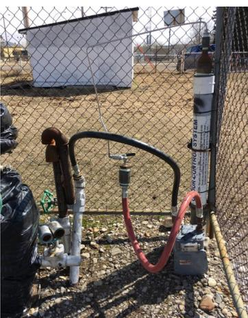
**Gas Migration Testing**— Surface test to determine if the casing has a gas leak that has migrated to surface through the ground.
