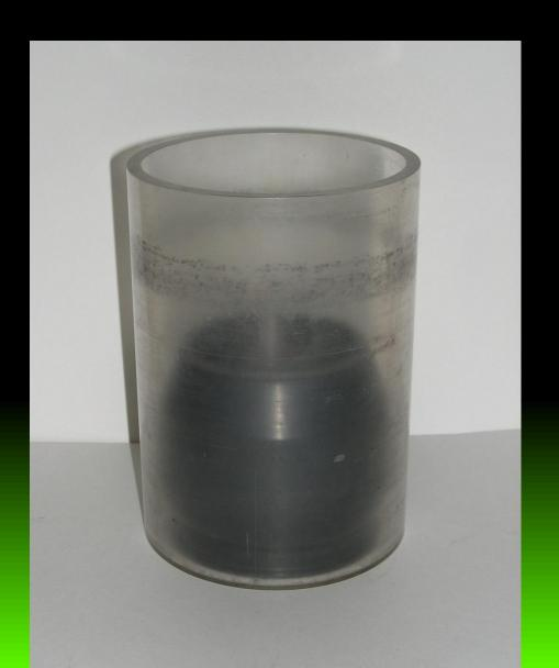
Lower Cup Profile showing expansion of major diameter due to weight of plunger compressing the ring at the bottom of the cup. Once the lower cup expands and seals with the casing wall, the upper cup then expands and seals by inflation due to pressure build up in the internal chamber of the plunger.
